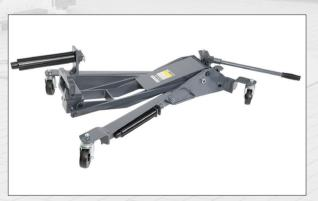
TQB Brands Borum Clutch Jacks use \* ISO32 hydraulic oil in their hydraulic ram and pump power packs to ensure compatibility with the seals used in their assembly.
