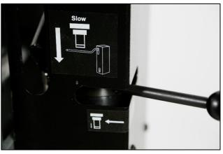
3. Insert the Pump Handle into the socket [slow manual pump] and pump the handle no less than twenty cycles.
