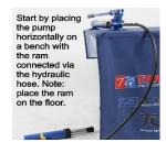
3. Turn the release valve clockwise to the lifting position.
